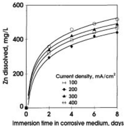
Fig. 1—Effect of current density on the corrosion resistance of Zn coatings in 3.5 wt percent NaCl at 0 rpm.
