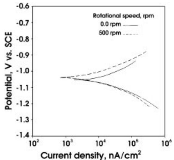
Fig. 5—Polarization curve for pure Zn coatings in 1-percent NaCl.
