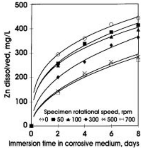
Fig. 3—Effect of specimen rotational speed on corrosion resistance of Zn coatings in 3.5 wt percent NaCl at 200 mA/cm<sup>2</sup>.
