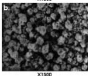
Fig. 7—SEM photographs of pure Zn coatings plated at: (a) 0 rpm; (b) 500 rpm; after immersion in 3.5 wt percent NaCl for 48 hr.
