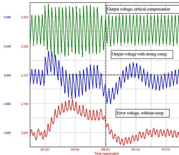
A close look at the error voltage response time leads to the closed-loop bandwidth of the SMPS. The measured rise time,  $t_r$ , is roughly  $22\mu s$ , which gives a bandwidth of:  $BW=1/\pi \cdot t_r = 14.5kHz$ , which corroborates our initial design goal value which was passed to POWER 4-5-6.
